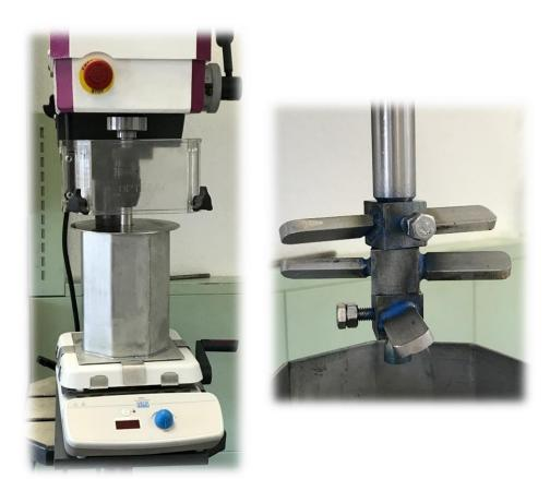
Figure 1: Attrition cell and stirrer - equipment for washing tests
